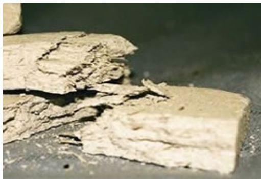
Pieces of Asbestos Insulating Board (AIB)
