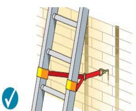
Tying near the base
